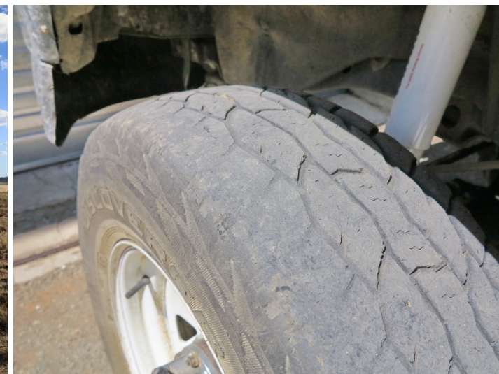
Fig. 6: Tyre worn smooth on the rocky tracks of NJF and TBP. We routinely run tyres down quickly (A. Sliwa).
